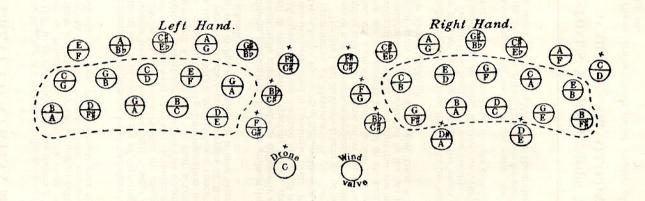
The upper notes marked on the keys are produced by compressing the bellows, and the lower ones by drawing the bellows out. For 30 keyed instruments the keys marked x are left out, and the keys of the 20 keyed instruments are contained within the dotted line. This sign  $\Lambda$  over a note indicates that the note is produced by drawing the bellows out.
